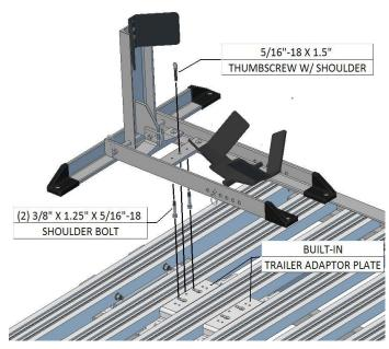
**Step 1**: Attach Shoulder Screws to the *CONDOR*® Pit-Stop/Trailer-Stop cross member as shown. (Torque parts A to 18 ft-lbs)
